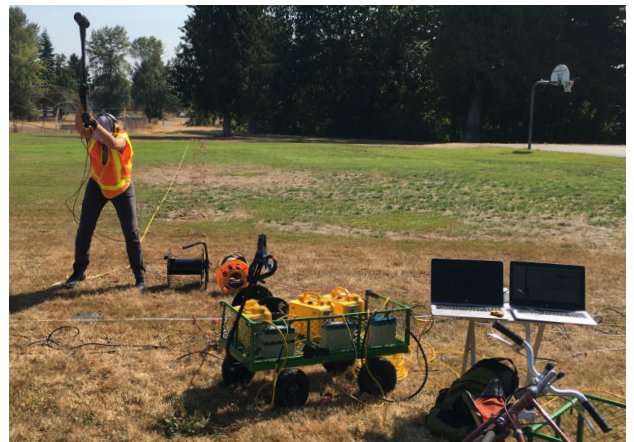
A WGS scientist generates seismic waves by striking a metal plate with a sledge hammer. The waves are recorded by an array of geophones visible on the ground in the background.
