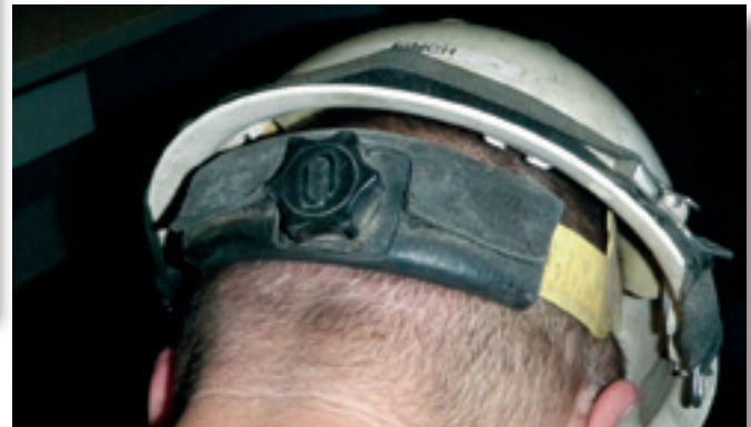
Figure 1—The sharp corners of the redesigned suspension system on the Bullard National Fire Protection Association (NFPA) 1977-compliant hardhats may cause discomfort.
