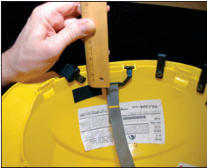
Figure 6—The two side tape strips need to be placed about 1 inch below the inner edge to clear the suspension attachment components.
