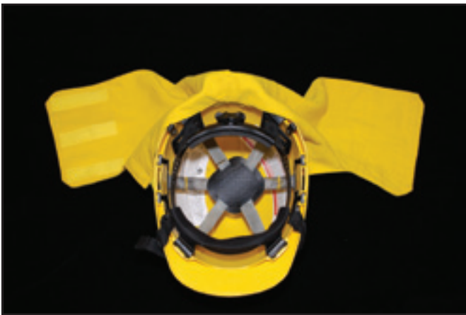
Step 2 —Attach the center loop tab (Velcro) of the shroud to the rear hook tape strip, stretch the sides around, and tuck the shroud material into the hardhat between the shell and the suspension system.
