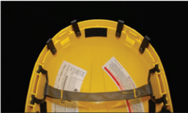
Step 1 —Place one tape strip horizontally inside the hardhat near the inner edge on the rear. Insert the suspension system into the hardhat.
