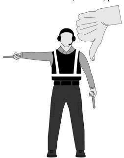
When responding to the flight crew request to connect external power, the parking tender will utilize the **Connect Power Hand Signal**.
