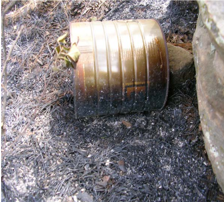
Figure 49. Example of advancing fire staining on a can.
