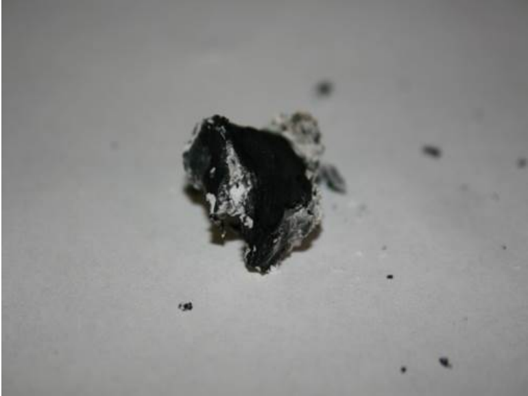
Figure 194. Remains of cardboard base from fusee.
