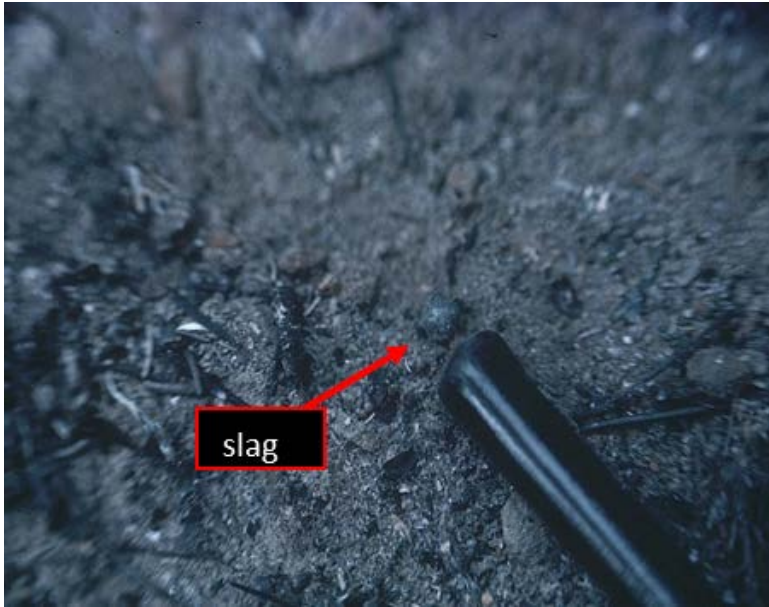
Figure 162. Slag located at the origin of a fire.
