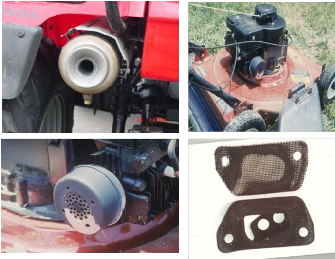
Figure 103. Several types of small engine exhaust systems.
