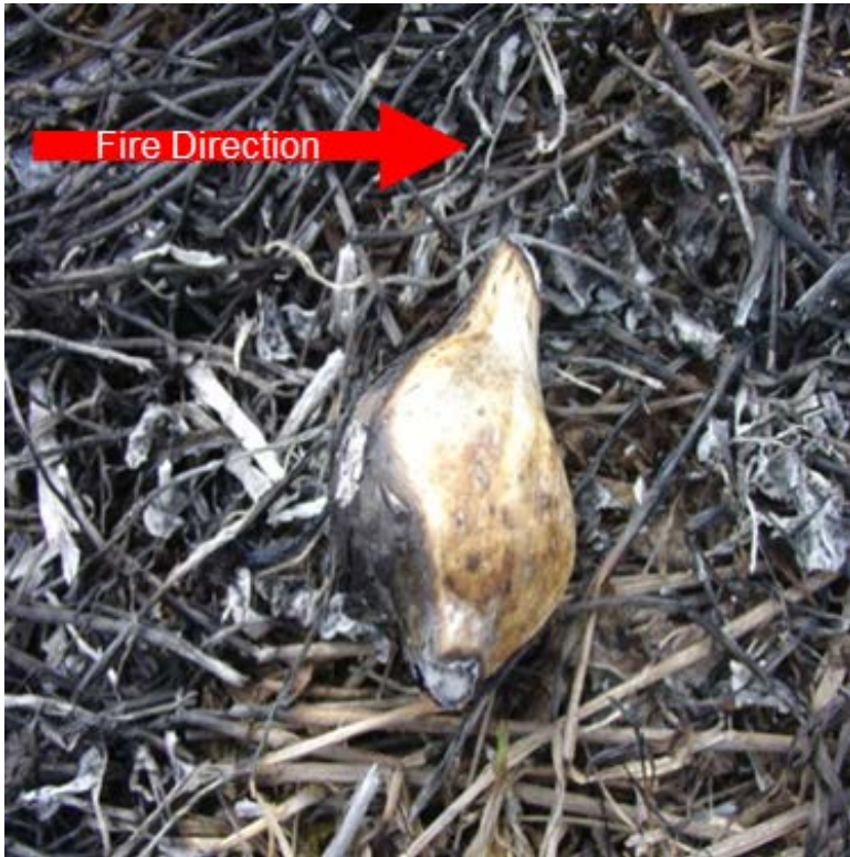
Figure 12. Example of microscale protection on smaller object that can be used to validate macroscale patterns.
