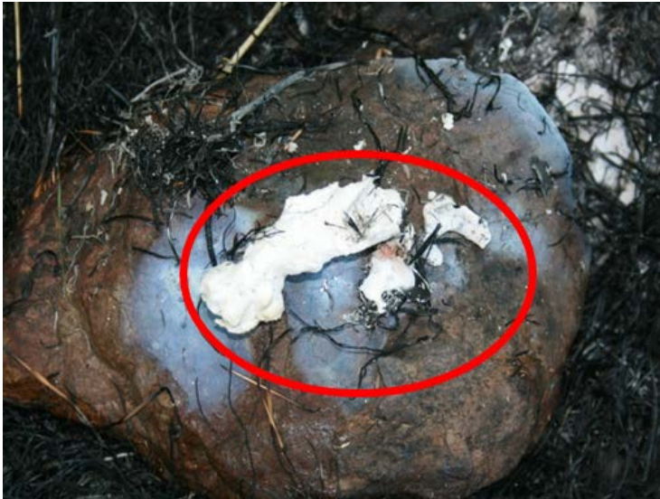
Figure 193. Slag from fusee on rock.
