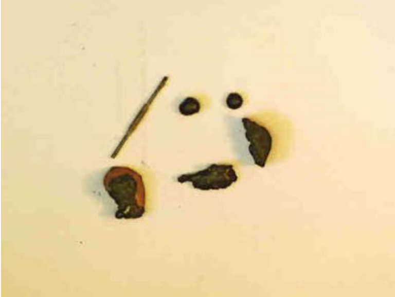
Figure 163. Welding by-products recovered from fire scene.
