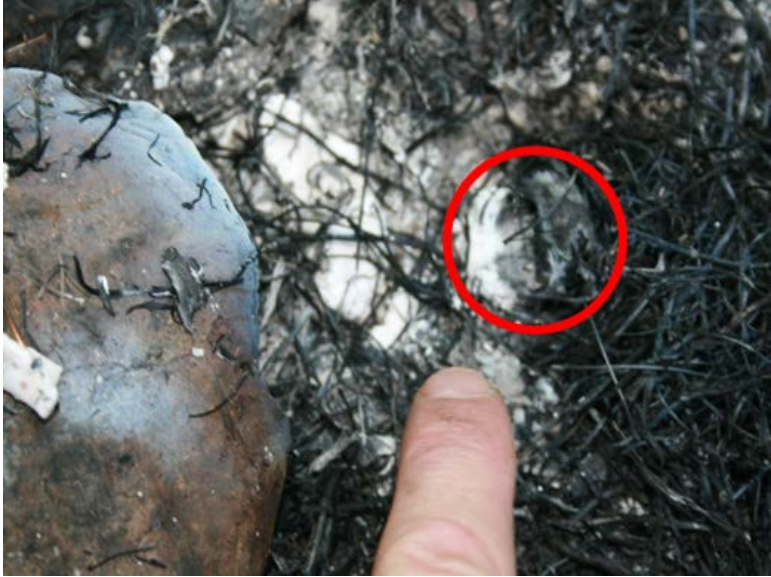
Figure 193. Slag from fusee on rock.
