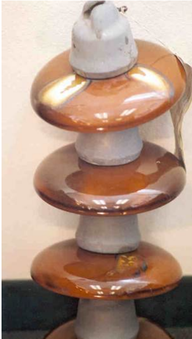
Figure 132. Arcing on a damaged insulator.
