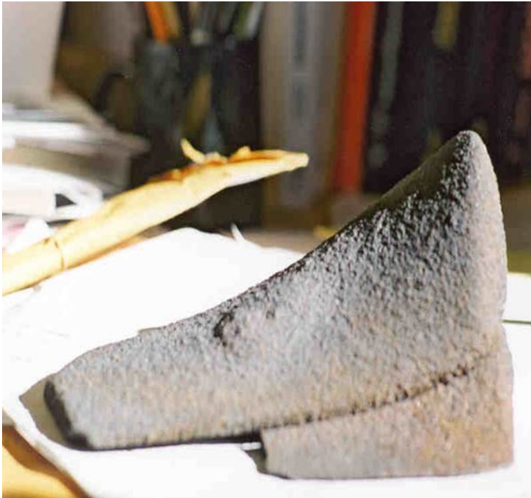
Figure 120. Track grinding slag.
