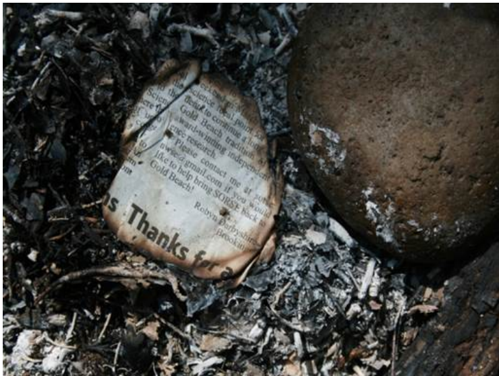
Figure 202. Paper remains protected under ignition device/rock.
