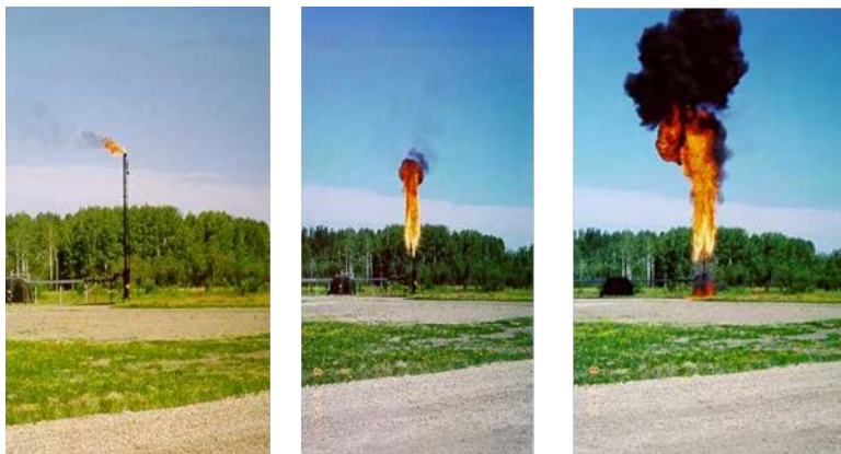
Figure 180. Flare stack malfunction leading to ground fire.
