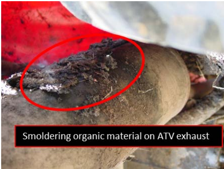
Figure 113. Conductive heat transfer ignition factor.
