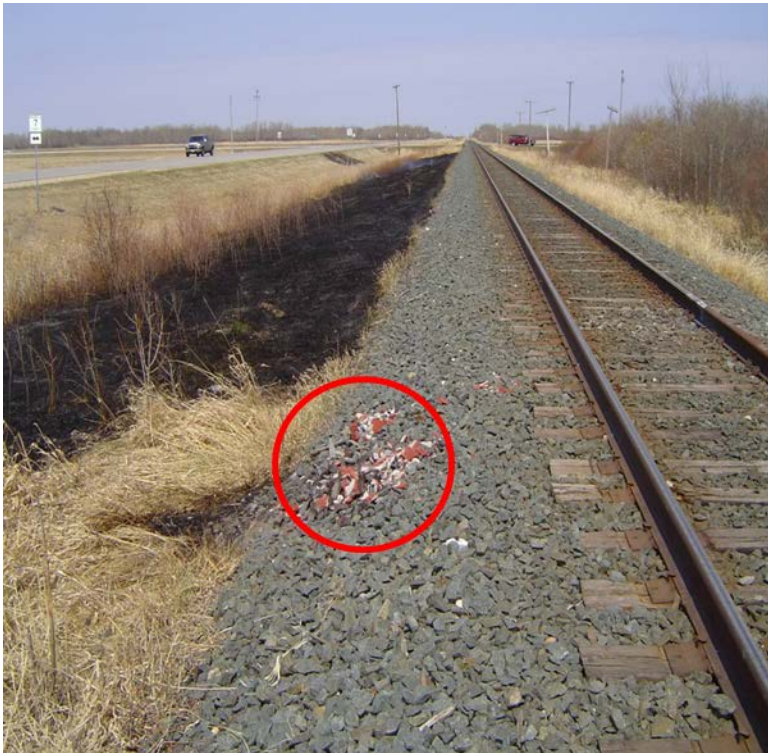
Figure 119. Ceramic molds along railroad track.
