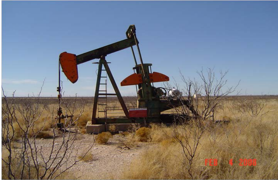
Figure 80: Pump jack on a shallow oil well
