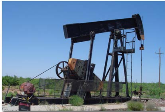
Figure 74: Oil well pumping unit with counter balance and electric motor
