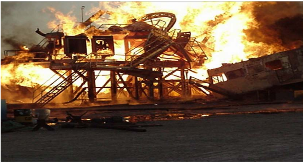
Figure 51: Blowout destroys drilling rig
