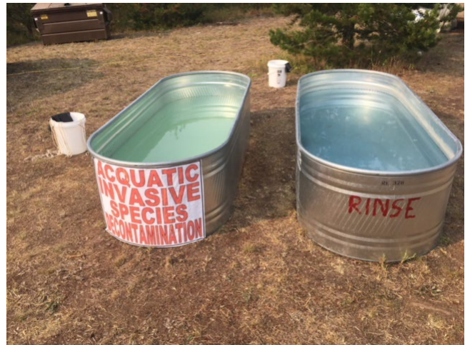
Figure 4: Example of a larger bath for longer/wider draft hoses
