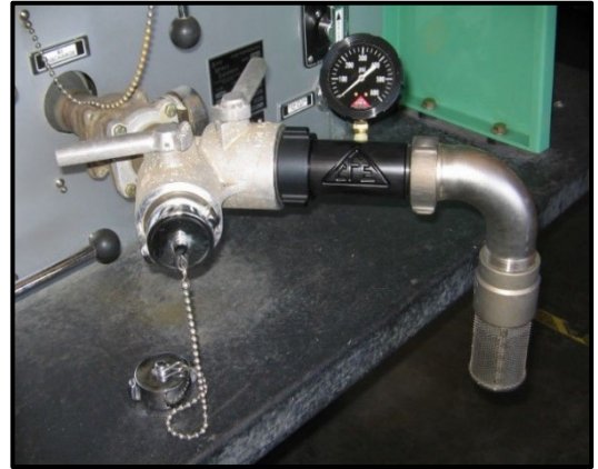
Figure 12: Pressure valve attached to the foot valve
