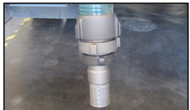
Figure 11: Foot valve attached to suction line with various adapters as needed to adjust for foot valve size
