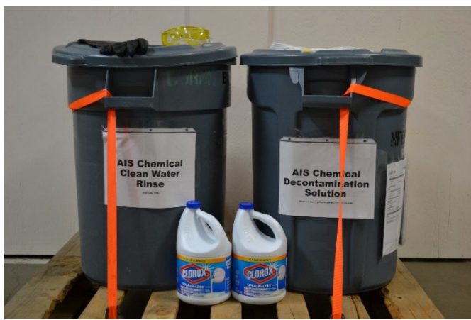
Figure 4: Chemical Decontamination Station Example
