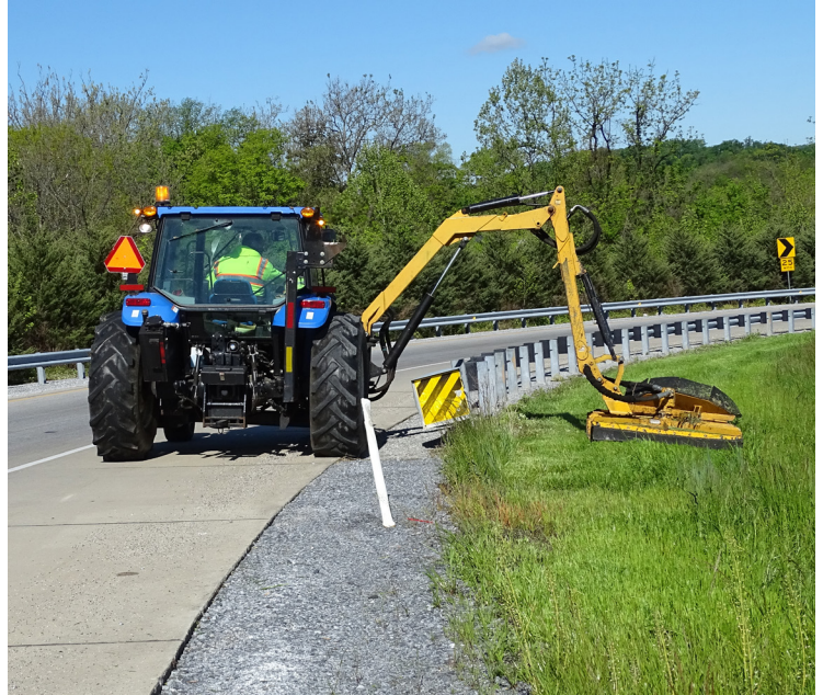
A boom arm mower being used in District 6 for roadside vegetation. Photo: PennDOT
