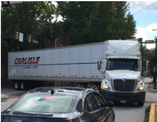
Figure 2: A truck encroaches upon an opposing lane in Mechanicsburg Borough. Photo: PennDOT LTAP
