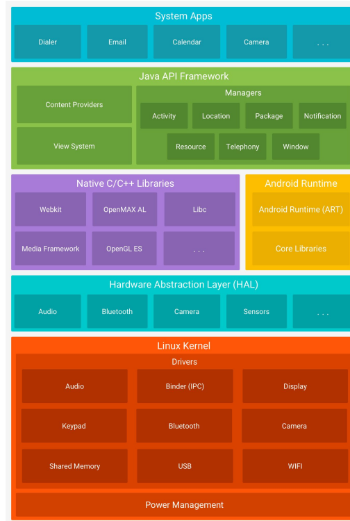
Diagram of Android OS internal layout
