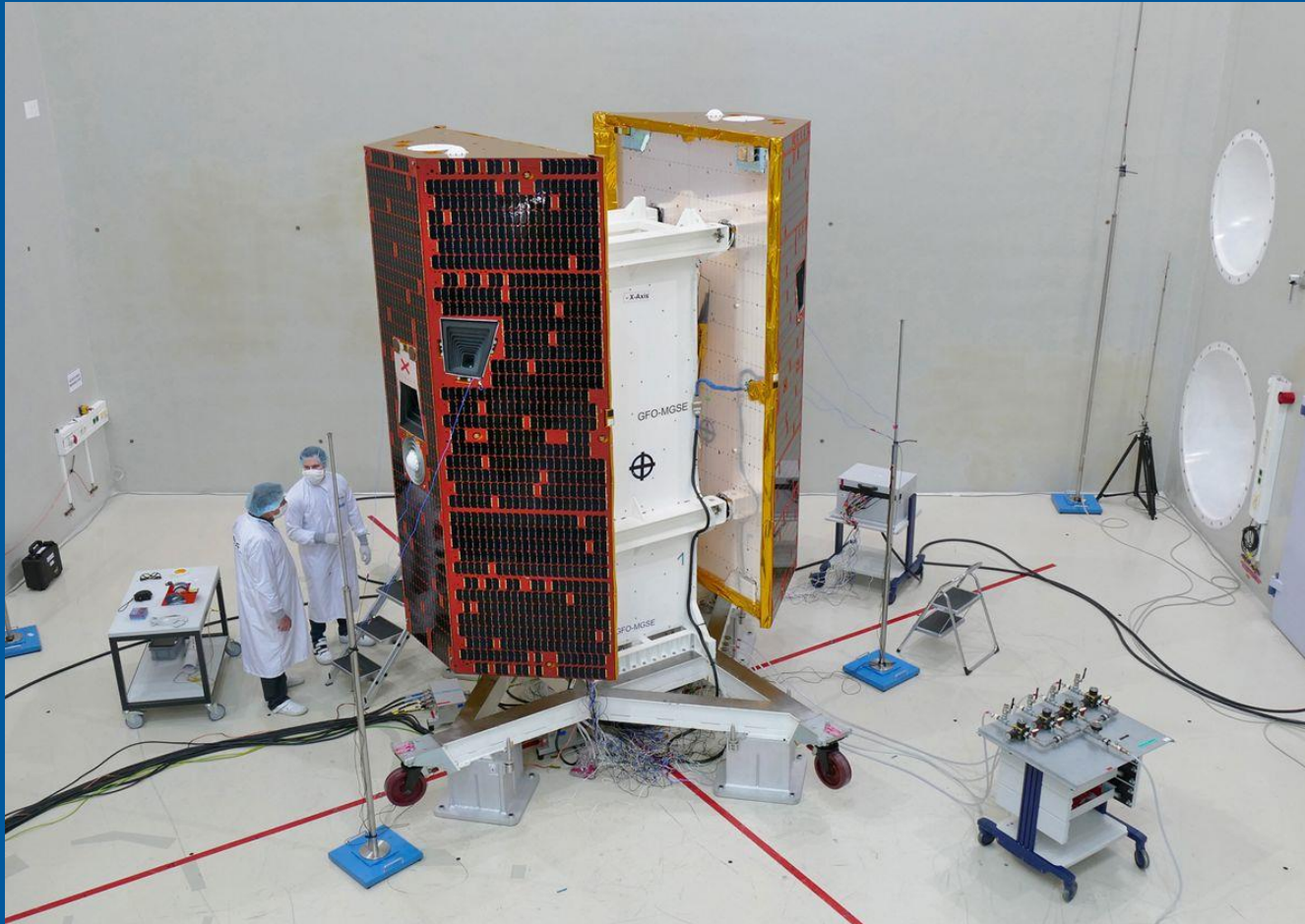
The GRACE-FO satellites prepared for acoustic noise test
