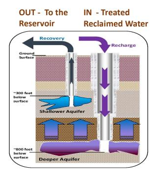
Under **one proposed alternative**, 50 mgd of highly treated reclaimed water would be injected 600-800 feet deep in the Floridan aquifer and pumped back up from shallower wells at 300 feet (see figure at left). 47 wells are projected to be used in the Seminole Heights area.
