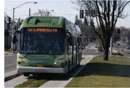
Above: Lane Transit in Eugene, Oregon, ran a six-month pilot of the PATH-developed automated guidance system for buses, which gave buses the efficiency of a light-rail system. Photo: Courtesy of PATH
