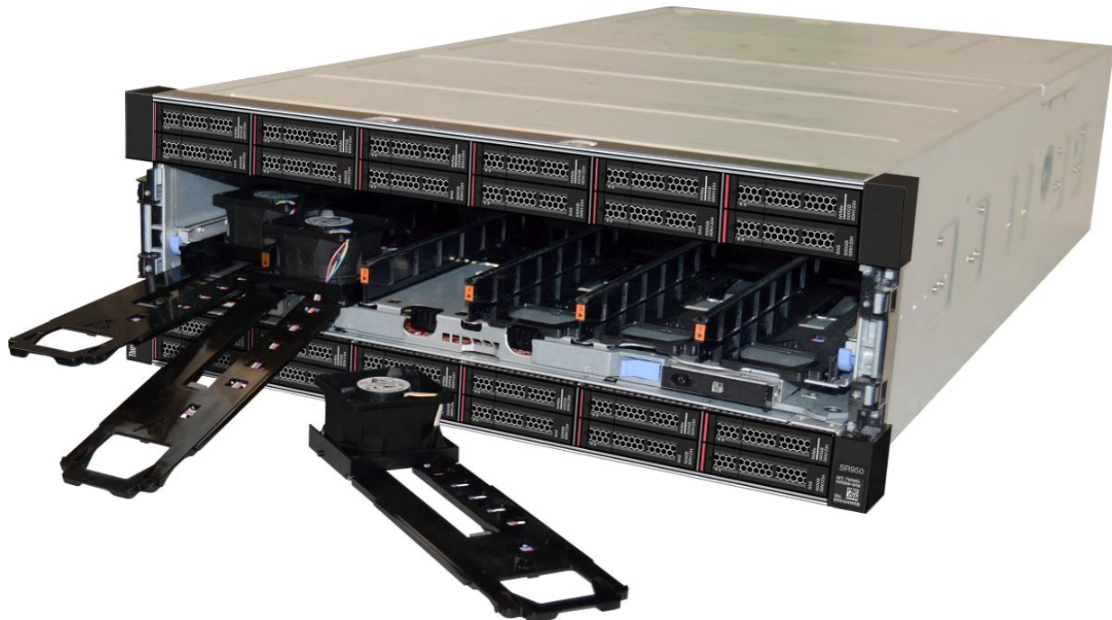
Figure 4. Fans are accessible from the front of the server
