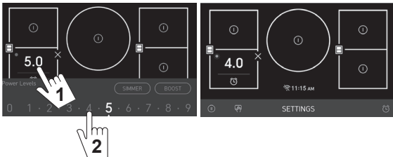
Readjusting power level 5 to 4
