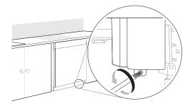
3 Use a Phillips screwdriver to remove 2 screws **1**.
