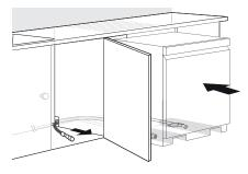
Remove the tape from the water supply line and the electrical cable.
