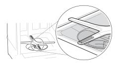
With the lower rack removed, place a level on the inside wall of the tub to check that the dishwasher is level from side to side.
