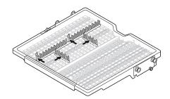
Pull tines back up to fit smaller dishes.
