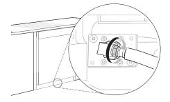
3 Slide the water supply line back through the channel, pulling gently from inside the cabinet to make sure the line is not kinked, pinched, stressed or crushed.
