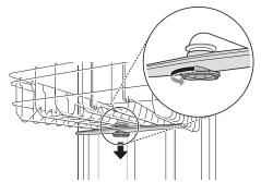
Remove food particles by rinsing or shaking the spray arm.
