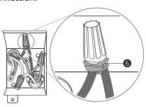
**10** Fold the connected wires back into the junction box and screw on the junction box cover.
