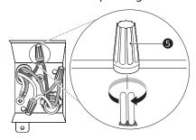
Wrap electrical tape **6** around each connection.
