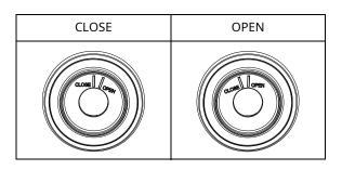
**5** For single-valve burners, insert a small, flatblade screwdriver into the valve stem. For dual-valve burners, insert a small, flatblade screwdriver into the hole to the left of the valve stem.
