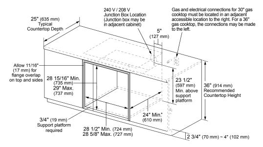
\*25" Min. (635 mm) cutout depth required for undercounter flush installation. Refer to installation art for flush installation in wall cabinet for required cutout dimensions.
