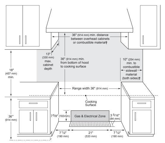
† as defined in the "National Fuel Gas Code" (ANSI Z223.1, Current Edition). Clearances from non-combustible materials are not part of the ANSI Z21.1 scope and are not certified by CSA. Clearances of less than 12" (305 mm) must be approved by the local codes and/or by the local authority having jurisdiction.
