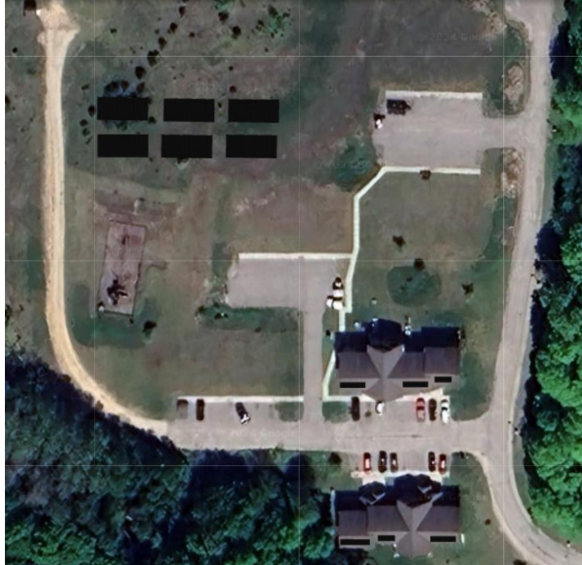
Image 1: A depiction of what the solar system at the Mtigwaakiis site could look like to offset current energy consumption after energy efficiency measures are installed (about 119 kW of solar).
