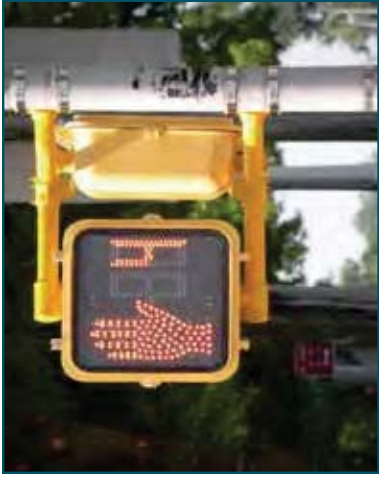
Pedestrian Countdown Signal Head
