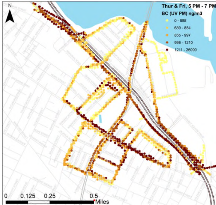
Figure 12: Spatial distribution of black carbon (BC) concentration during evening rush hour (5-7 PM) on weekdays (Th-F). Each data point represents the average of all measurements in all three seasons within 50-m x 50-m grid cells.
