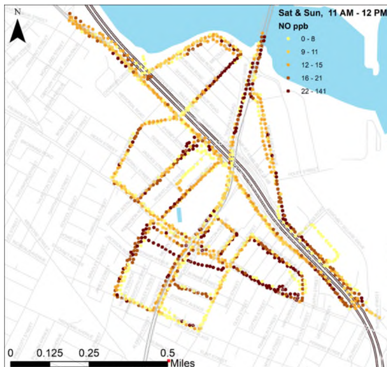
Figure 15: Spatial distribution of nitric oxide (NO) concentration during midday rush hours (11 AM - 12 noon) on weekends (Sa-Su). Each data point represents the average of all measurements in all three seasons within 50-m x 50-m grid cells.
