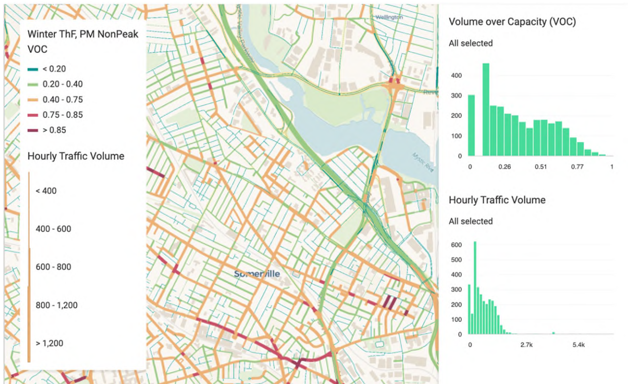
Figure 21: Estimated Traffic Volume and Volume over Capacity (VoC) for PM Peak Hour and Non-Peak Hour on Thursdays and Fridays for Winter (Jan, Feb, 2019)
