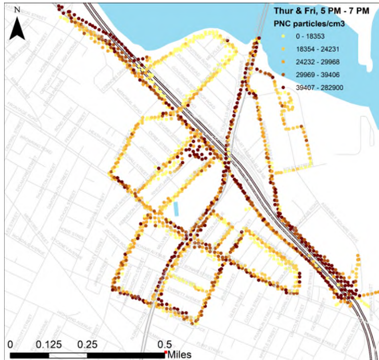
Figure 10: Spatial distribution of particle number concentration (PNC) during evening rush hour (5-7 PM) on weekdays (Th-F). Each data point represents the average of all measurements in all three seasons within 50-m x 50-m grid cells.
