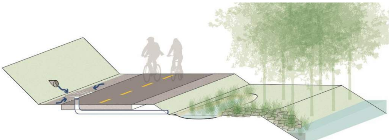
Figure 22. Stormwater Management Schematic at existing outfalls
