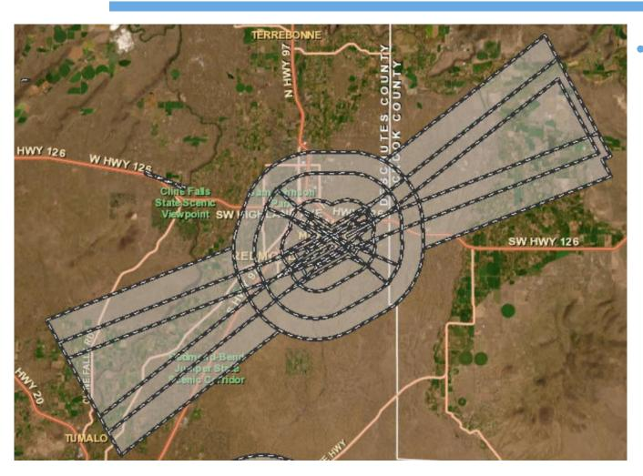
"Imaginary areas in space and on the ground that are established in relation to the airport and its runways. Imaginary areas are defined by the primary surface, runway protection zone, approach surface, horizontal surface, conical surface, and transitional surface." (Oregon Dept. of Aviation model code definition)
