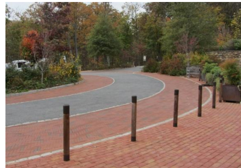
Though no curbs are used, the bollards and change in materials communicates where cars can drive or stand and which zone is for pedestrians.
