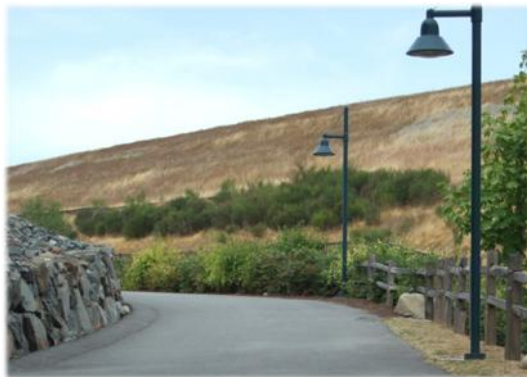
Trail lighting that is scaled for pedestrians and bicyclists. Frequent fixtures create a uniform lighting level.
