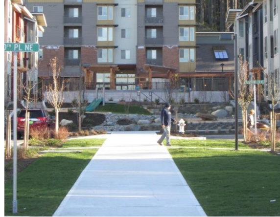
This central pedestrian spine uses consistent materials and stays at a constant grade, even when crossing roads. Though this walkway crosses a road, just past the person, the road is secondary to the walkway so it is difficult to detect in the photo.
