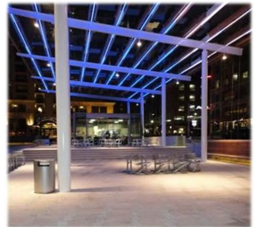
LED lights in the pavillion and plaza allow changing colors at night, creating an engaging element. In the lower image, the area under the pavillion is lit to a higher level than the rest of the plaza since this is the area most likely to be used at night.
