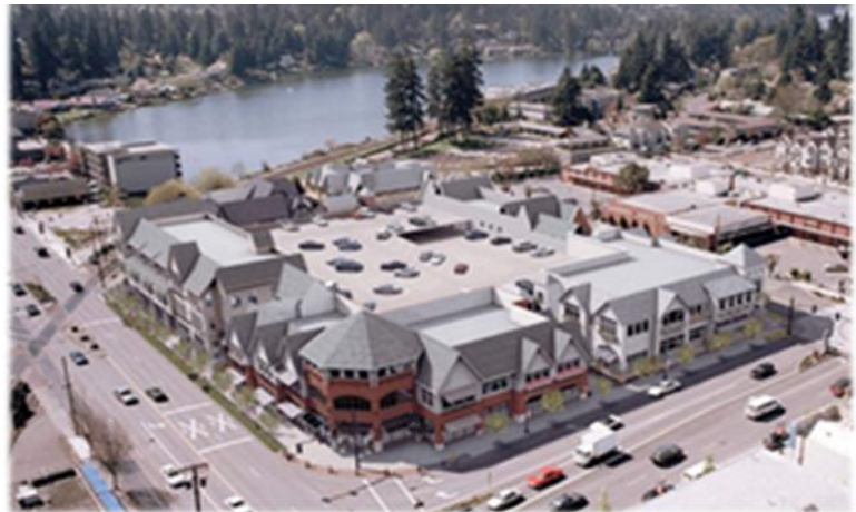
This aerial view shows active uses wrapping a structured parking garage, eliminating its impact on the Circulation facilities and pedestrians.
