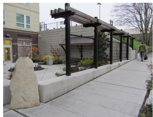
Where a streetwall isn't present, but is needed, this technique provides a visually permeable edge to both sidewalk and adjacent plaza.
