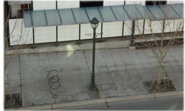
The street trees and lights have been coordinated, ensuring good lighting and no conflicts with trees. This much separation is not necessary in all circumstances.
