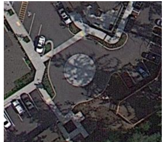
Contrasting pavement has been used to both identify important pedestrian crossings and also to direct vehicular movements. The circle can be driven over by fire trucks, but tends to slow private cars who drive around it.
