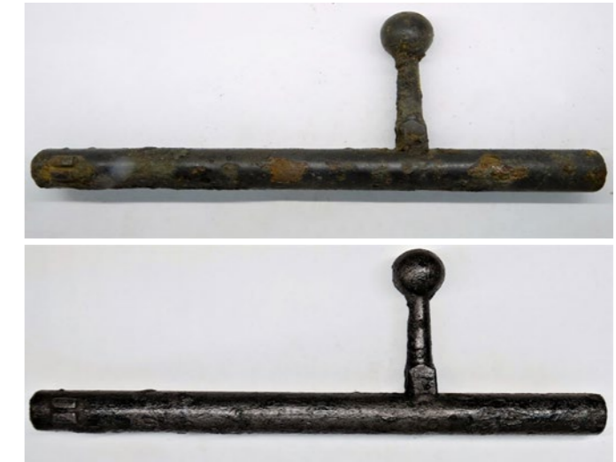
◀ IMAGE PROTECTIVE INSERT WZ. 1933 FOR MAUSER RIFLE WZ. 98A; BEFORE AND AFTER CONSERVATION
