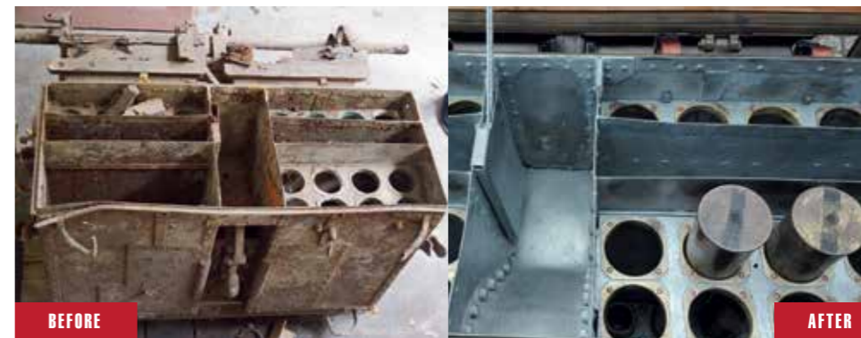
Ammunition box and tubes of the field gun caisson before and after conservation. Photo: Marcin Westphal
