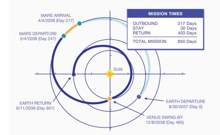
**Trajectory and timeline for a typical "opposition-class" mission to Mars, the baseline mission considered in this report.** *Due to the changing orbital positions of Earth and Mars, an opposition-class mission would involve a shorter stay on Mars (30 to 90 days) and a shorter total mission time (400 to 750 days) than the alternative "conjunction-class" mission. SOURCE: NASA, Human Exploration of Mars, Design Reference 1045 Architecture 5.0, p. 48.*
