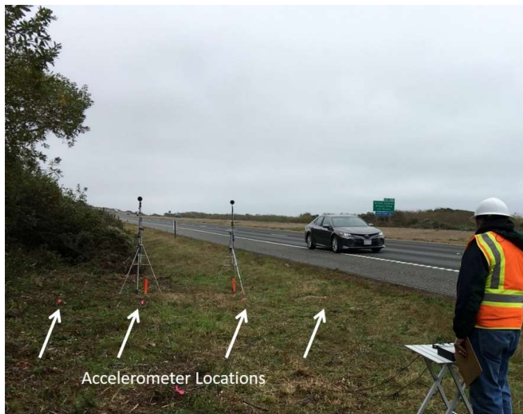
Figure B-16: Ground vibration accelerometers installed at the mumble strip pass-by site
