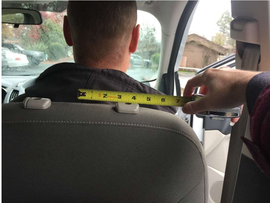
Figure B-11: From the center point between the headrest holes, the microphone was positioned 5 inches outward
