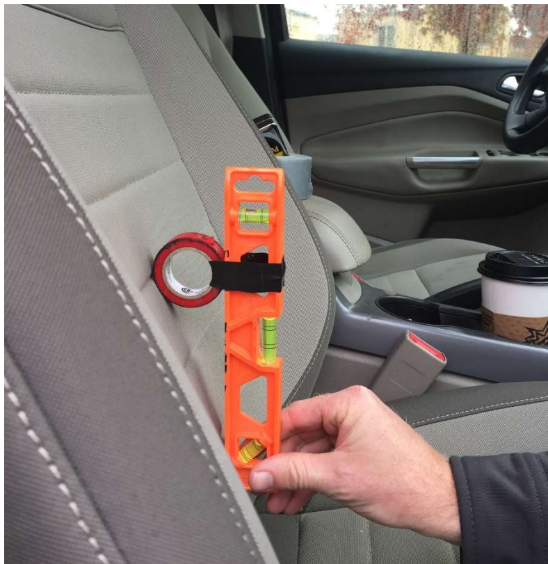
Figure B-7: Device fashioned in field to measure the 19-degree angle of the seat back
