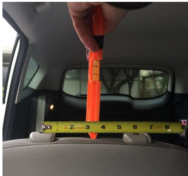
Figure B-8: Determine the center point between the two headrests
