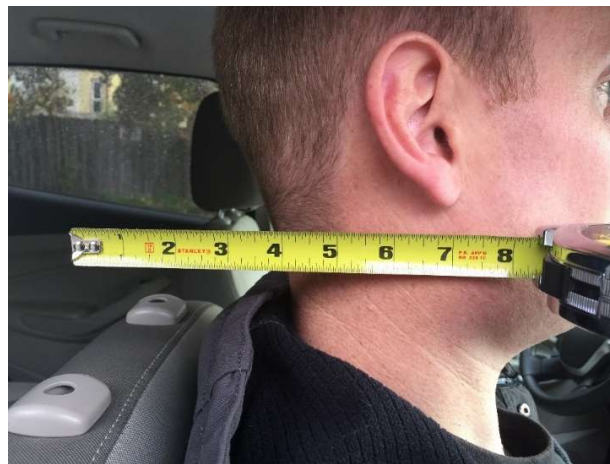
Figure B-9: For the average male passenger, the ear is located approximately 7 inches from the center of the headrest holes
