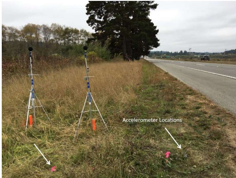
Figure B-17: Ground vibration accelerometers installed at the conventional rumble strip pass-by site
