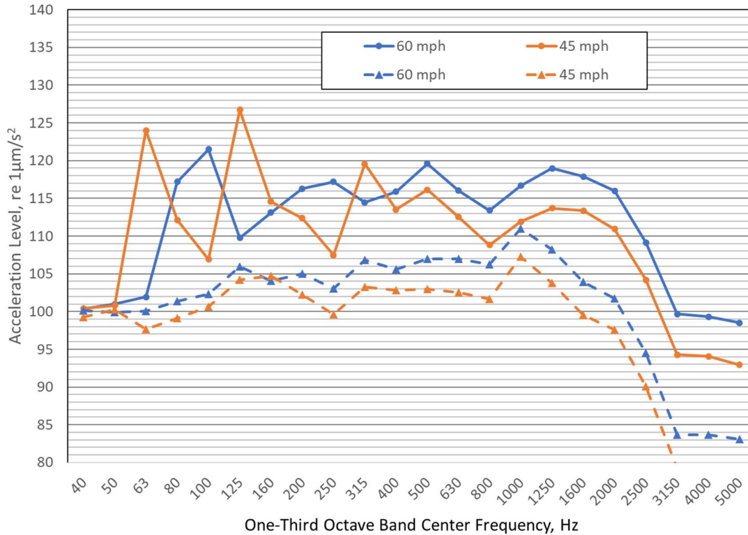
Figure B-112: One-third octave band spectra for the summed seat track locations on conventional ground strips at 45 and 60 mph for Test Car 4
