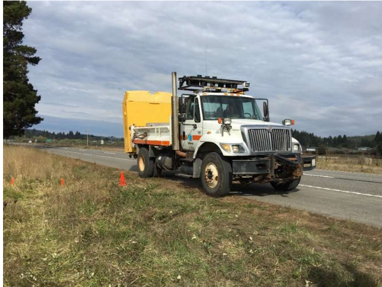
Figure B-15: Caltrans 4-yard dump with mounted barrier
