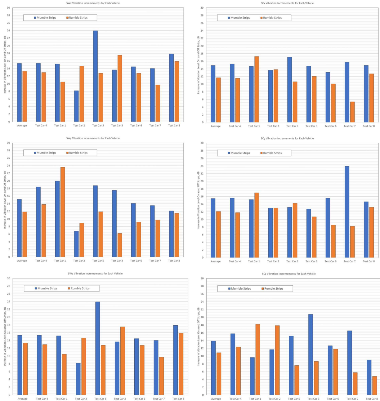
Figure B-91: Difference in level on and off the mumble and conventional ground strips for all vehicles in each direction at locations related to steering wheel and column, SWx, SWy, SWz, SCx, SCy, and SCz
