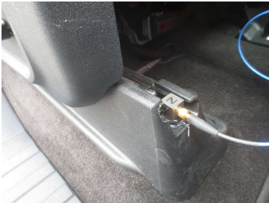
Figure C-13: Triaxial accelerometer installed at the seat track location
