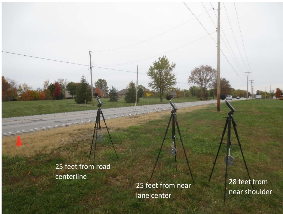
Figure C-12: Typical sound level meter arrangement for shoulder and centerline rumble strip pass-by noise measurements
