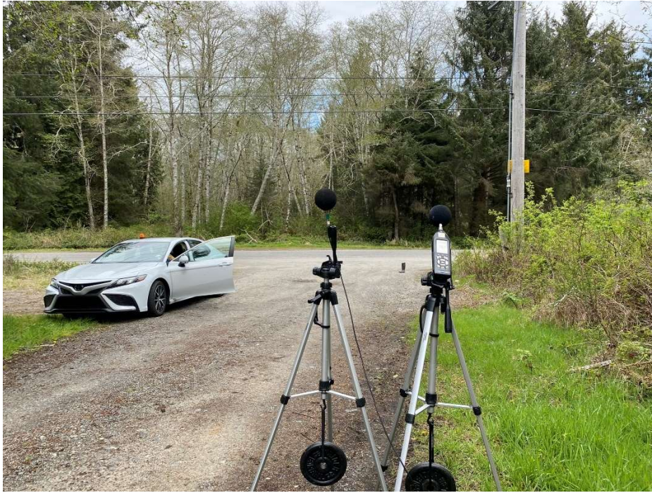
Figure D-34: Microphone location 153 feet from 16-inch sinusoidal strips at Site WB2
