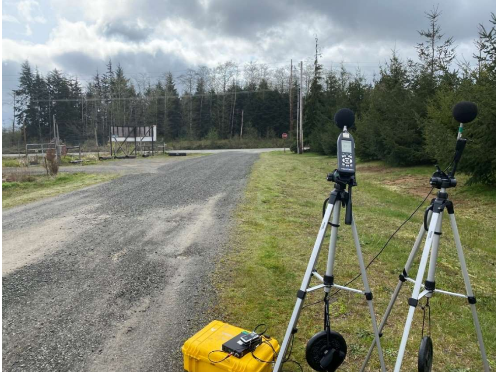
Figure D-29: Microphone locations at 234 ft from EB1 sinusoidal strips
