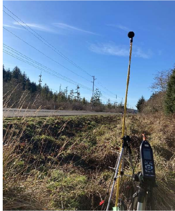
Figure D-7: Examples of microphone placements to be 5ft above pavement surface
