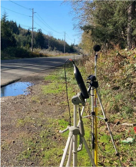
Figure D-7: Examples of microphone placements to be 5ft above pavement surface
