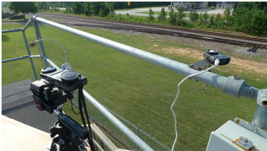
Figure 9: Horizontal illuminance equipment: CLTC illuminance meter with shading disk (left) and Velux illuminance meter (right)
