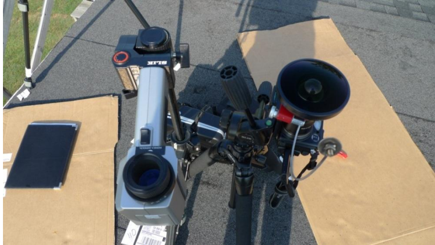
Figure 8: Sky luminance equipment: Luminance meter (left) and HDR camera for (right)
