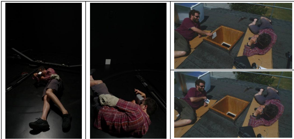
Figure 14: Measurement of the reflectance of the interior walls of the goniophotometer room and the light well panels
