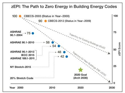
The Zero Energy Performance Index (zEPI) is a relative scale that allows various levels of building energy performance to be compared against each other. zEPI sets an energy use intensity (EUI) target for building type and is adjusted for climate. This graph charts zEPI scores for the current national model energy codes and standards.
