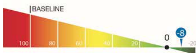
Figure 15. The Zero Energy Performance Index (zEPI). The NZE Certified Omega Center for Sustainable Living in Rhinebeck, NY has a zEPI score of -8.
