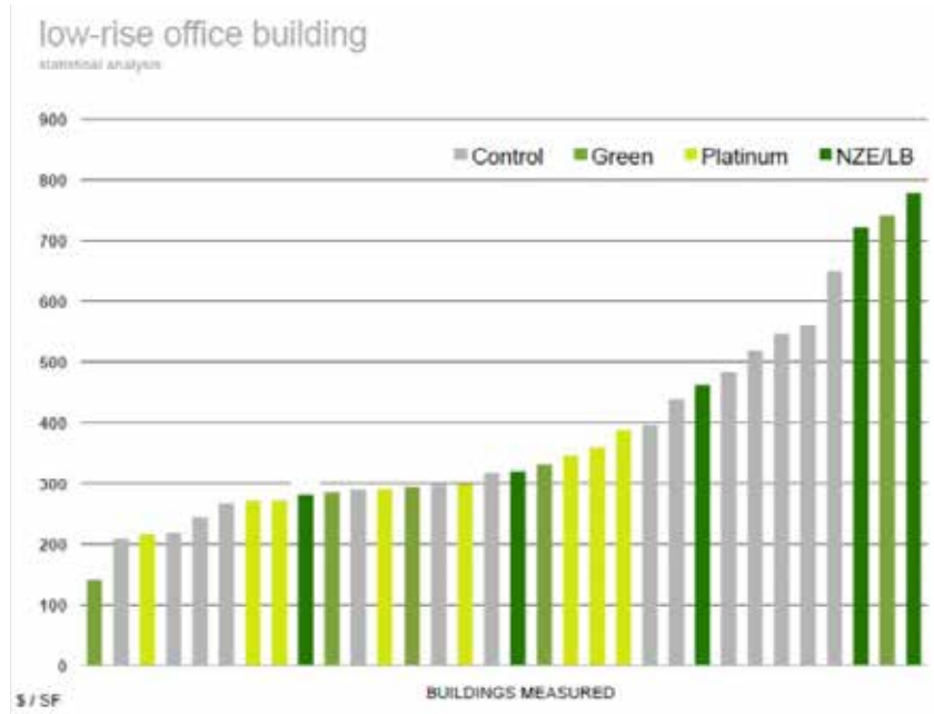
Figure 3. Comparison of Total $/Sf of Standard, Green, LEED Platinum, and NZE Buildings. Integral Group’s analysis showed that deep efficiency doesn’t have to come at a cost premium. Green, LEED Platinum, and NZE projects were delivered at costs comparable to the control group. Credit: Integral Group, 2018.
