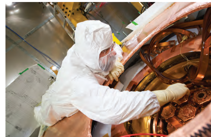
The Super Cryogenic Dark Matter Search uses towers of disks made from silicon and germanium to search for particle interactions from dark matter.
