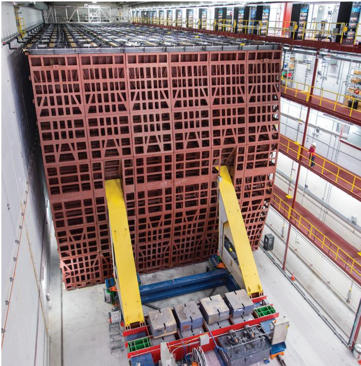
The NOvA detector in Minnesota occupies an area about the size of two basketball courts. It is 200 feet long and made of modules 50 feet high and 50 feet wide. The detector records particle tracks from neutrinos sent by a powerful accelerator at Fermilab. The construction of the NOvA detectors was completed in the fall of 2014, on time and under budget. The experiment is scheduled to collect information until 2025.
