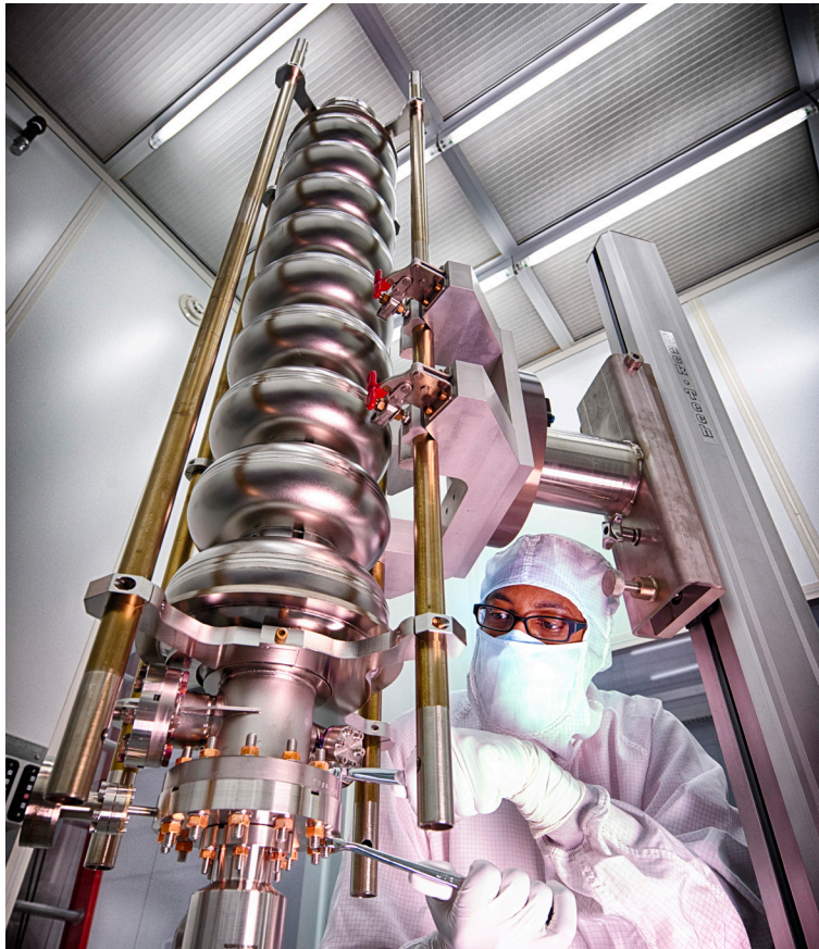
SRF acceleration cavities such as this one accelerate particle beams. Fermilab scientists and engineers conduct extensive research to make the cavities as efficient as possible.
