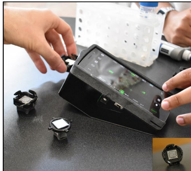
A multiplexed biomarker sensor that is quantified and read through a mobile phone for patient testing in clinical settings and even at home. Credit: Ozcan Lab at UCLA.
