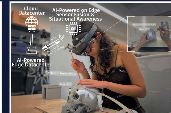
NSF Athena's augmented reality-assisted neurosurgical system provides guidance to surgeons, enhances the accuracy of surgical tasks and maximizes patient safety. Photo credit: Maria Gorlatova, Duke University.
