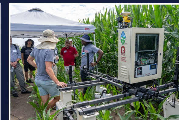
AIIRA Robotics Team demonstrating the use of robotics for sensor placement in a corn fields. Photo credit: USDA-NIFA AIIRA.
