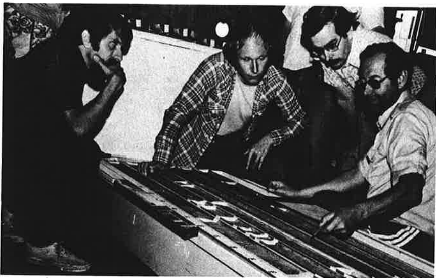
Deep Sea Drilling Project. Scientists aboard Glomar Challenger , operating in the Atlantic Ocean south of the Bermuda Rise, examine basalt recovered from a deep hole drilled under more than 5 kilometers of water. Penetrations like this, which drill nearly a kilometer below the ocean floor, provide important data for understanding the structure of ocean basins.
