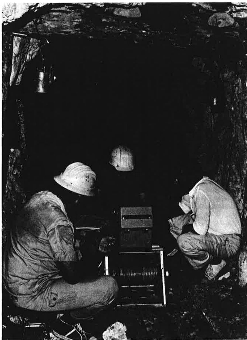
Special Foreign Currency project. Egyptian and American scientists (from Southern Methodist University) measure borehole temperatures in the Abu Dabbab Mine in the eastern Egyptian Desert to study heat flow in the continental crust. The region around the Red Sea is drawing scientific interest as a possible embryonic spreading center splitting Africa from Arabia. (Photo by Paul Morgan, SMU)
