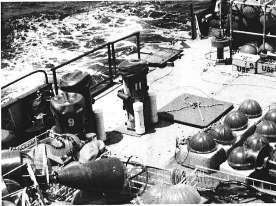
Sediment traps. The photo at the left shows parts of a floating trap that catches ocean particles over a wide path and at varying depths. At right is a larger, cone-shaped trap; these and other designs were used in a comparative experiment in the Panama Basin. Sediment traps, which can also be moored, help oceanographers understand the rate at which particles form, sink, or dissolve. Scientists then know more about the composition and chemistry of seawater and sediment on the ocean bottom.
