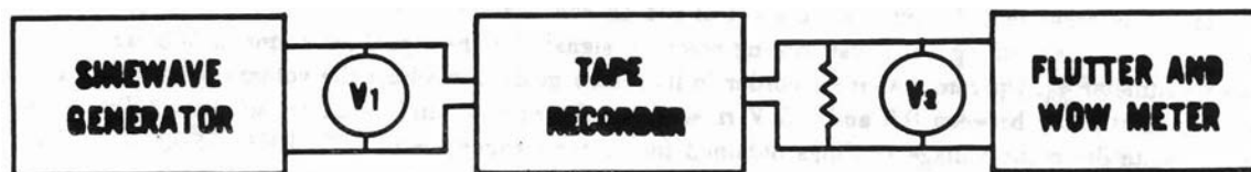
FIGURE 8. Block diagram for the weighted peak flutter and wow measurements.
