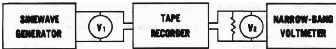
FIGURE 7. Block diagram for the system distortion, power amplifier distortion, input dynamic range, adjacent-channel cross talk, and record input voltage measurements.
