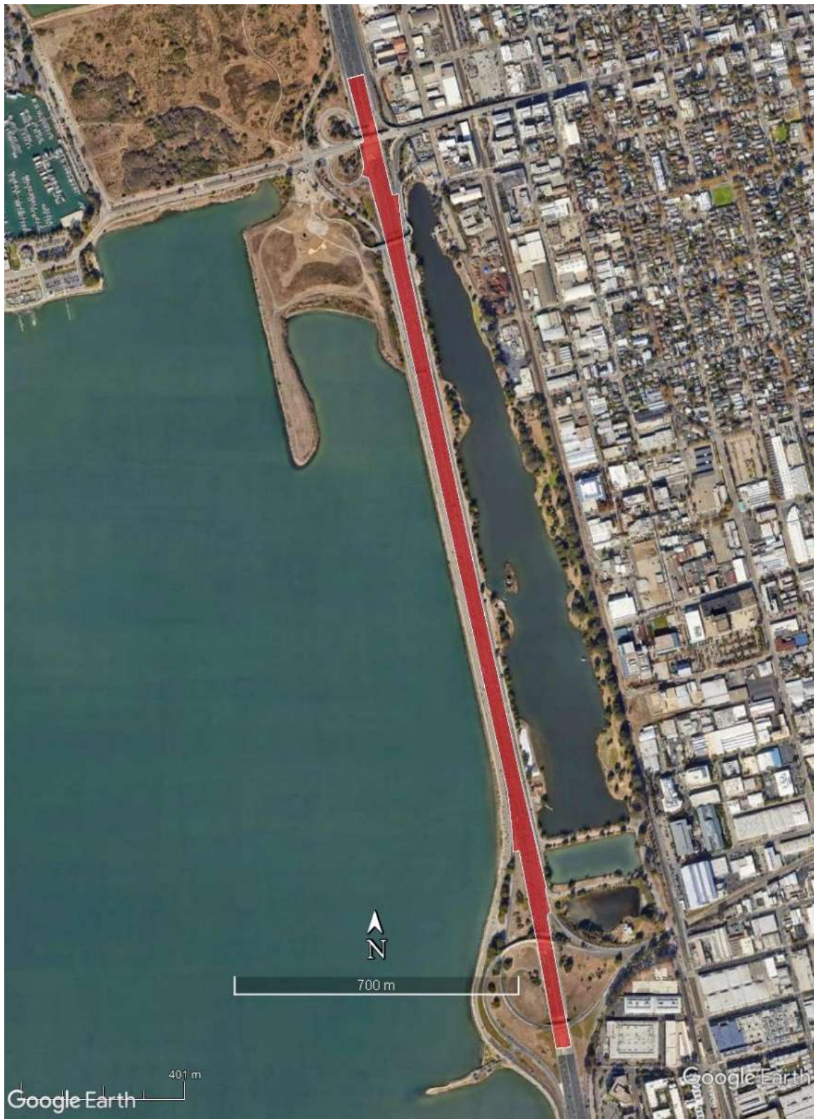
Figure 2-1. "Areapoly" source geometry used in tracer-based evaluations (with AERMOD)
