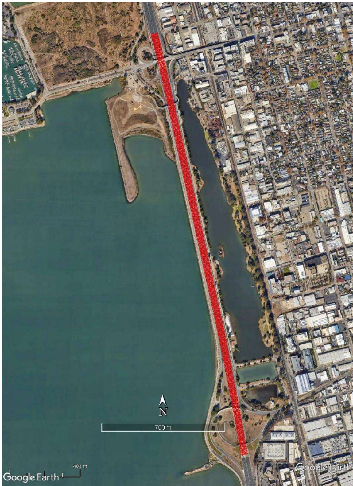
Figure 2-5. Volume source geometries used in tracer-based evaluations (with AERMOD)
