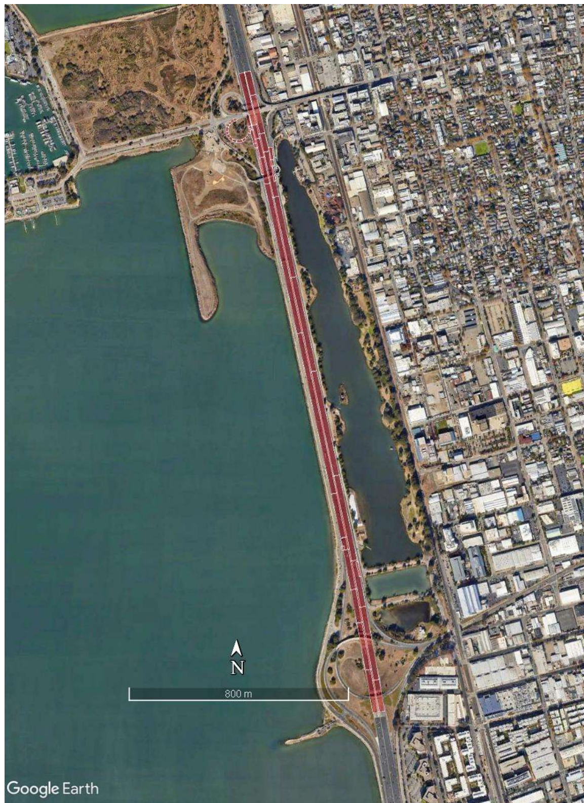
Figure 2-10. Line source geometries used in pollutant- and regulatory-based evaluations (with CAL3QHC)
