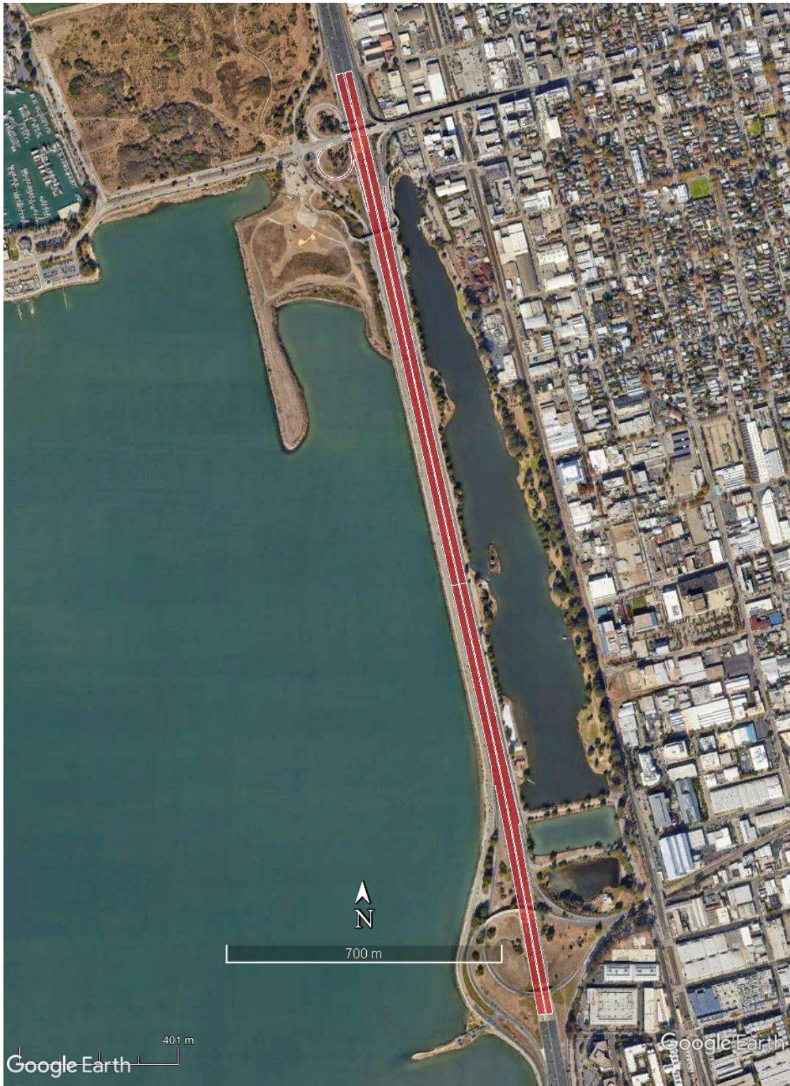
Figure 2-3. "Areapoly" source geometries used in pollutant- and regulatory-based evaluations (with AERMOD)
