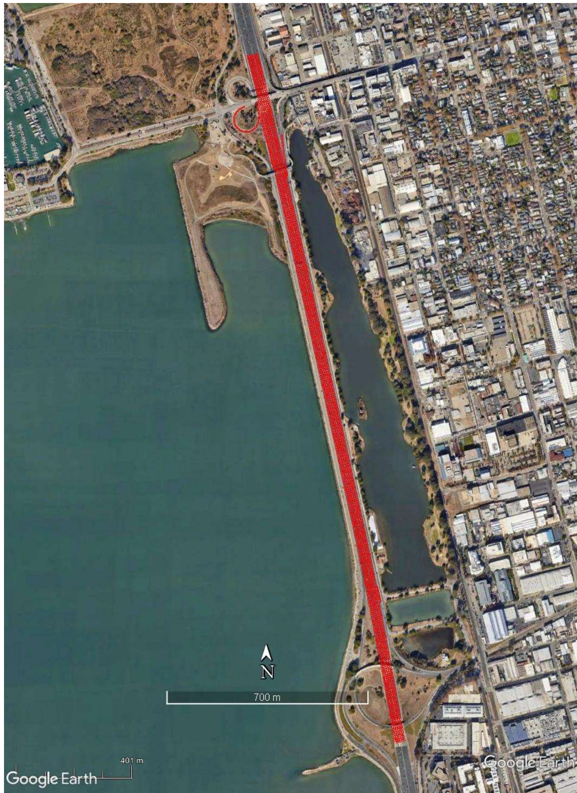
Figure 2-6. Volume source geometries used in pollutant- and regulatory-based evaluations (with AERMOD)
