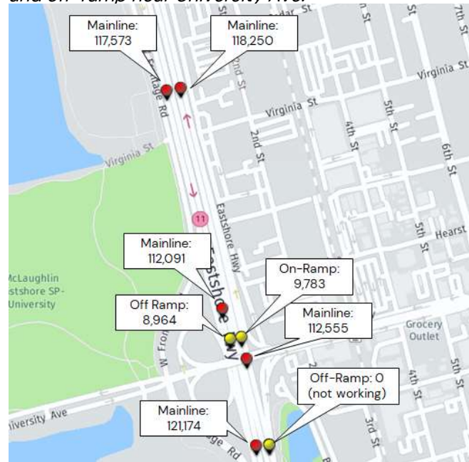
Figure 4-9. Traffic counts on mainline as well as on- and off-ramp near University Ave.
