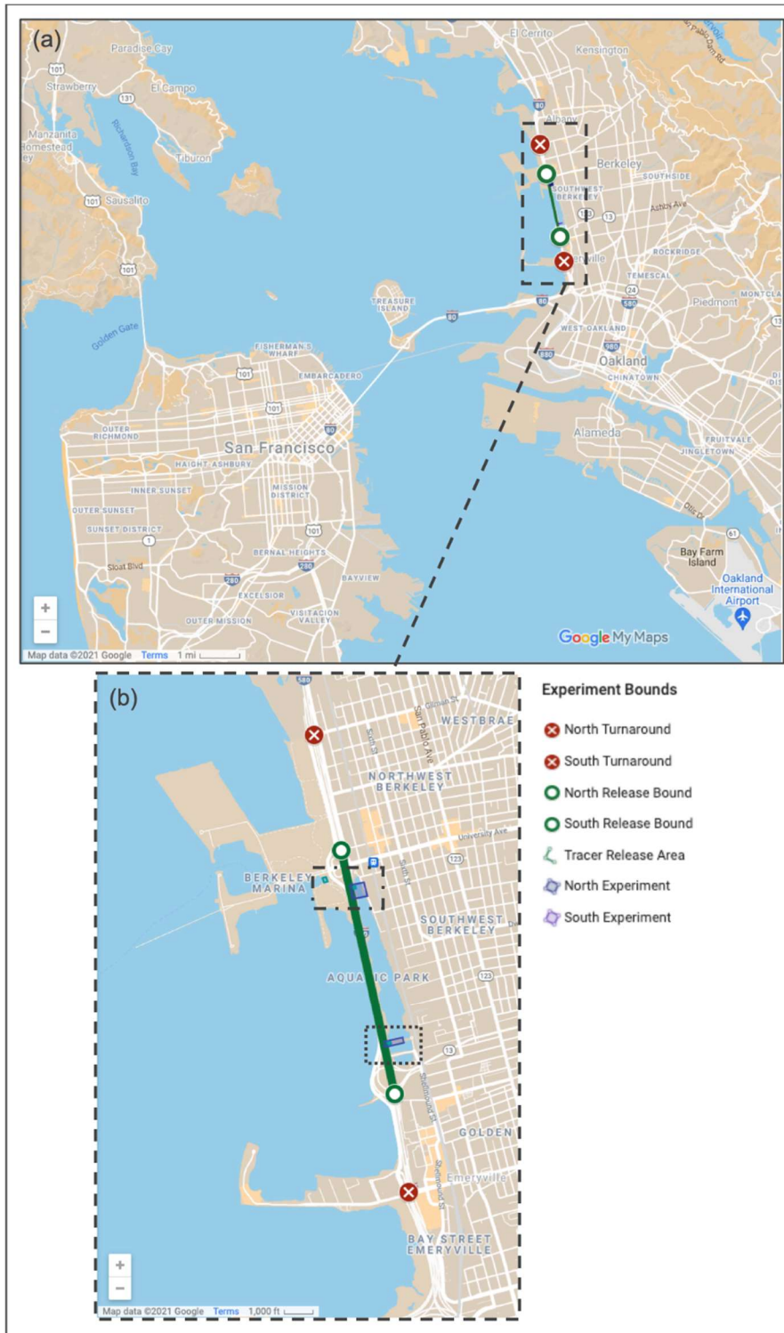
Figure B-1. The study area along I-80 in Berkeley, CA, with greater detail for the boxed area indicated in (a) shown in subpanel (b). The mobile platform turnaround points are marked by the red circles with a white X and the tracer release zone is shown by the green line bounded by the open green circles. The two experimental areas noted by the two boxes in (b) and shown in greater detail below in Figure B-2. Maps are from Google and oriented vertically north-south, with scale noted in the lower left text box of each subplot.
