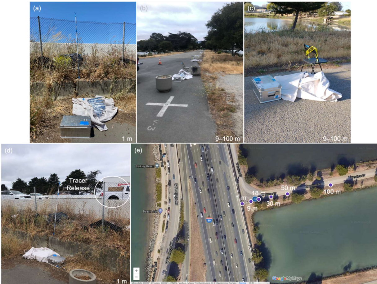
Figure B-3. In the South Aquatic Park Experimental Area, samplers were placed at downwind target distances of 1, 9, 18, 30, 50, and 100 m. The inlet height at the 1 m distance (a) was extended to a height about 3 m above the sampling area ground level, while the inlets of all other samplers were elevated to about 0.7 m on the backs of folding chairs (b, c). Note the passing mobile tracer release platform in (d) relative to the elevated inlet for the nearest highway sampler also shown in (a).
