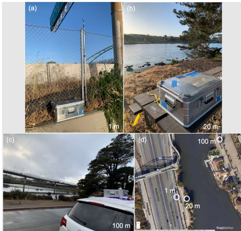
Figure B-2. North Experimental – North end of Aquatic Park, Berkeley, CA. Tracer gas samplers were placed at downwind target distances of (a) 1, (b) 20, and (c) 100 m. All inlet heights were >1 m above ground and were placed away from potential obstacles that would bias sampled air flow.
