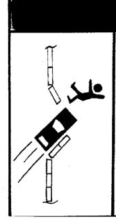
When pinned together, this product is classified as a longitudinal channelizing device (LCD), NOT a positive barrier. Like plastic traffic cones, this device is intended to serve as a visual channelizing device to direct vehicles or pedestrians. This device is NOT designed to keep vehicles penetrating through. DO NOT use longitudinal channelizing devices in applications where people or fixed objects are intended to be protected from vehicle impacts.
