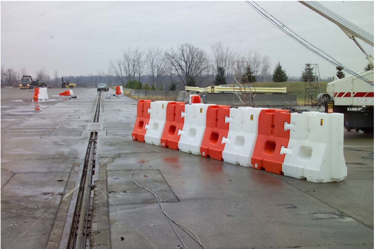
Figure A-43 Post-Test Channelizing Barricade Impact Side Downstream Overall - View 2
