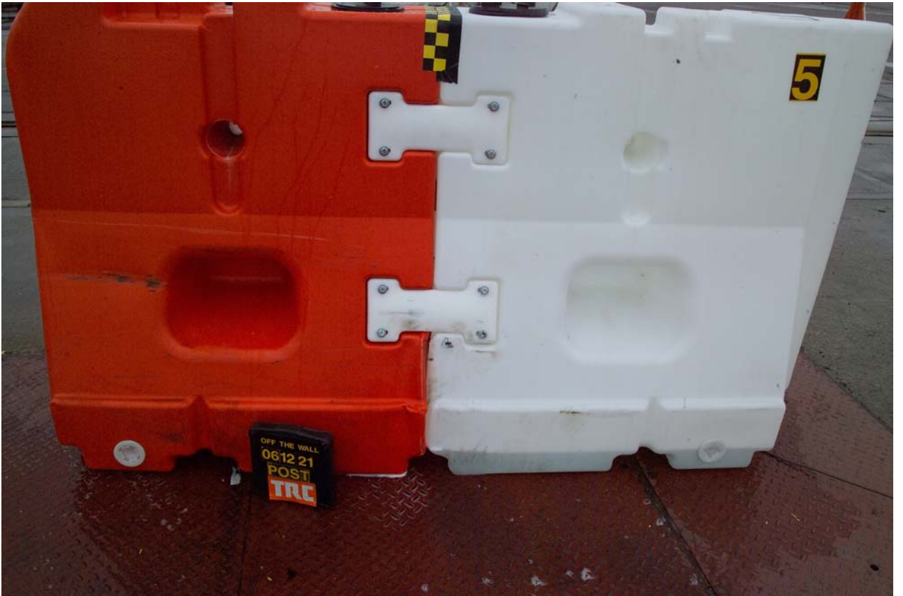
Figure A-61 Post-Test Damage to Barricade 5 - View 1
