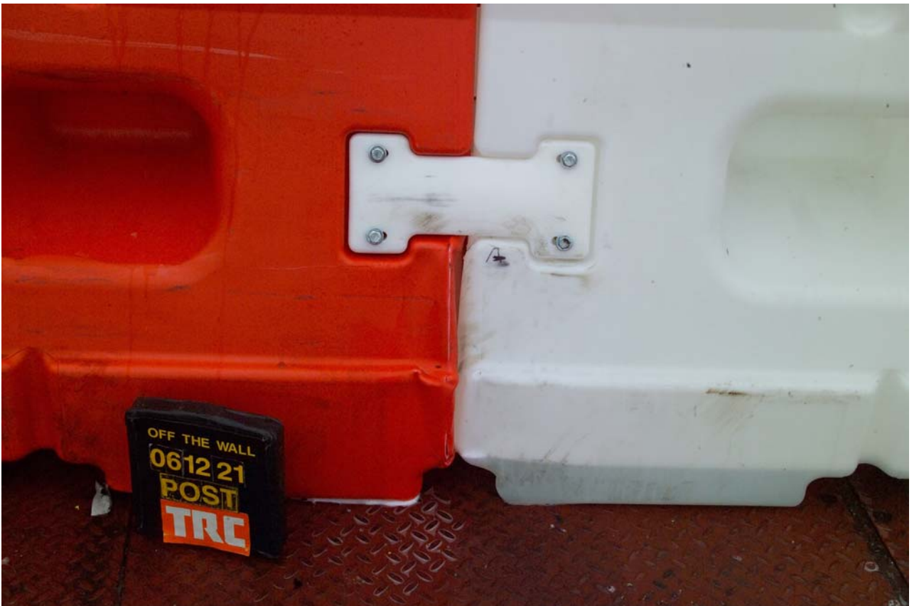
Figure A-62 Post-Test Damage to Barricade 5 - View 2
