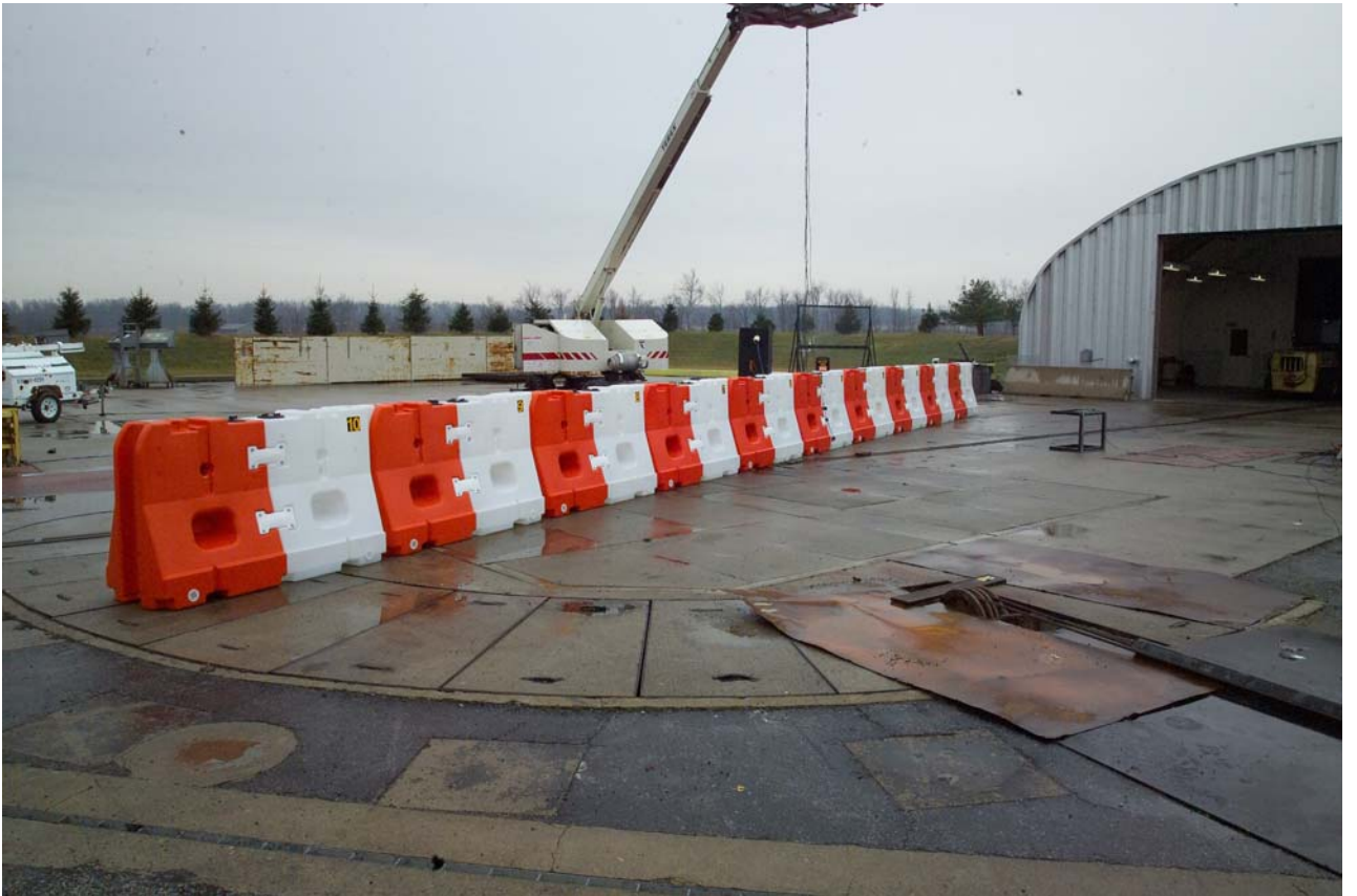
Figure A-36 Pre-Test Channelizing Barricade Impact Side Upstream Overall View
