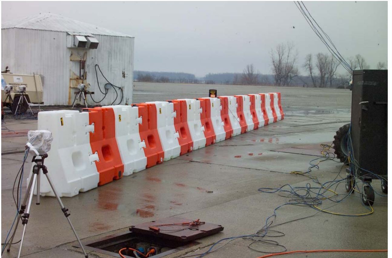
Figure A-46 Pre-Test Channelizing Barricade Non-Impact Side Downstream Overall View
