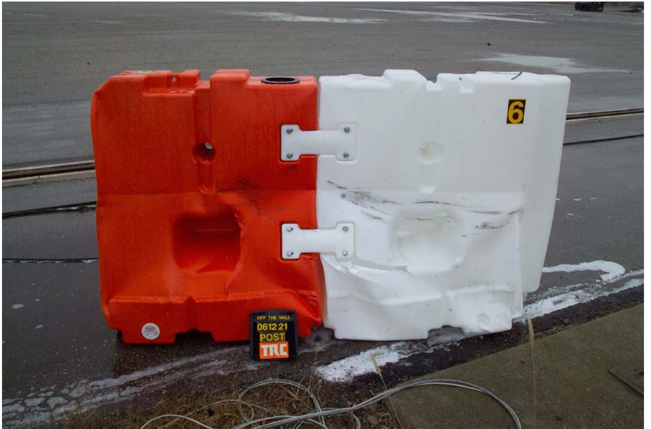
Figure A-63 Post-Test Damage to Barricade 6 - View 1
