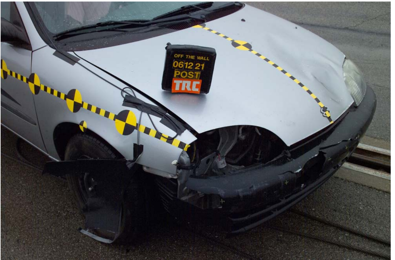
Figure A-18 Post-Test Vehicle Damage - View 2
