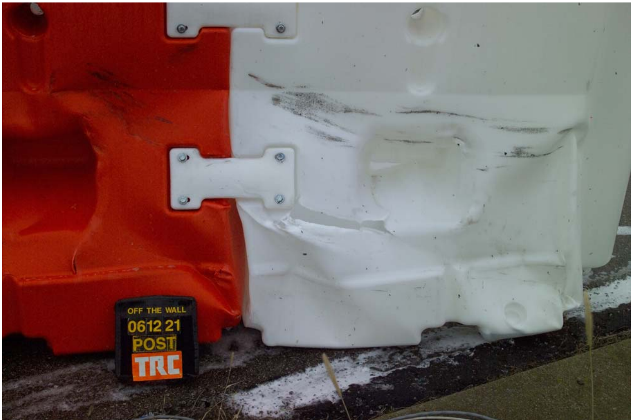
Figure A-64 Post-Test Damage to Barricade 6 - View 2
