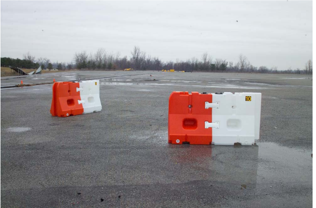
Figure A-70 Post-Test Channelizing Barricade Resting Position - View 5
