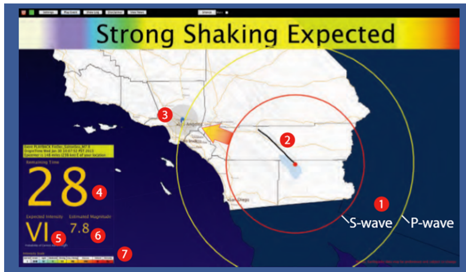
Figure 4. ShakeAlert computer message for a magnitude 7.8 scenario earthquake on the southern San Andreas fault. It shows the number of seconds before seismic shaking waves arrive at a location, the expected shaking intensity at that site, and a map with the earthquake epicenter, its magnitude, and the current position of the P and S waves. (Source: USGS, ShakeAlert—An Earthquake Early Warning System for the United States West Coast, Fact Sheet 2014-3083)
