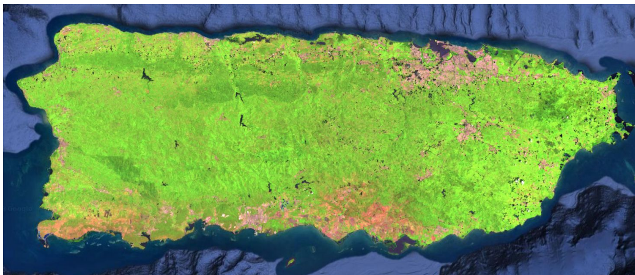
Fig 2a -- Pre-Maria Landsat 8 false-color image with display colors red as band 6 (SWIR), green as band 5 (NIR), and blue as band 4 (red).
