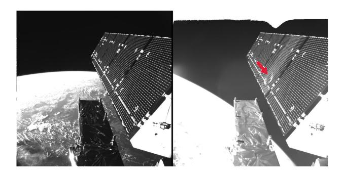
The picture shows Sentinel-1A's solar array before and after the impact of a millimetre-size particle on the second panel. The damaged area has a diameter of about 40 cm, which is consistent on this structure with the impact of a fragment of less than 5 millimetres in size. Credit: European Space Agency
