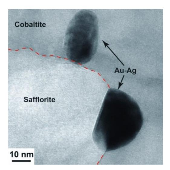
Close-up of the melting of two gold nanoparticles. The one on the right is under melting process, while the one on the top has already melted completely and has taken on a fully rounded shape. Credit: University of Barcelona
