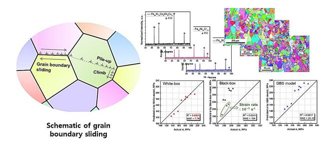
Schematic of grain boundary sliding and experimental validation and model comparison for various iron-based alloys. Credit: POSTECH
